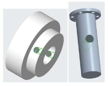
Figure 05 and 06: Actuator pulley CAD model created in Creo
