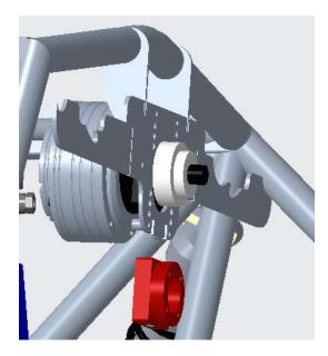
Figure 11: Creo model of the autonomous steering system with all components.
