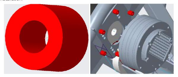
Figures 09 and 10: Actuator mounting assembly with spacers, CAD rendering created in Creo.
