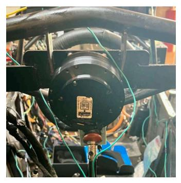
Figure 15: Back view of the actuator, parallel to the driving column
