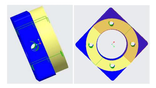
Figures 07 and 08: Steering column pulley and its mounting support, CAD models created in Creo.
