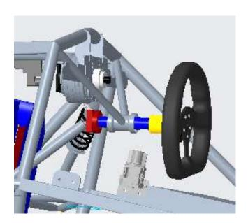
Figure 04: Pulley mechanism of the AK10-9 KV60 actuator, illustrated using the Creo CAD model
