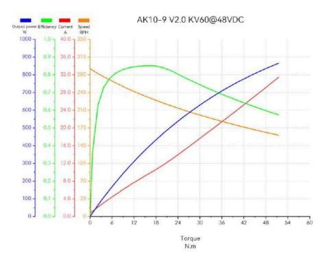
Figure 03: Graph of current, speed, efficiency, and power as a function of torque, obtained from the official <u>CubeMars AK10-9 V2.0 KV60 product page.</u>
