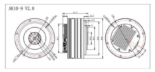
Figure 01: Technical drawing sourced from the <u>CubeMars AK10-9 V2.0 KV60 product page</u>.
