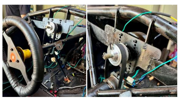
Figure 13 and 14: Front view of the actuator installation showing the belt drive connection and mounting plate configuration.
